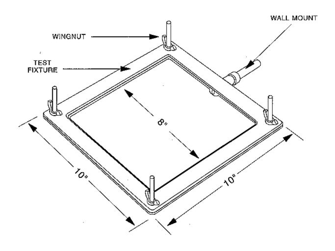
FIGURE B-4. HORIZONTAL TEST FIXTURE
