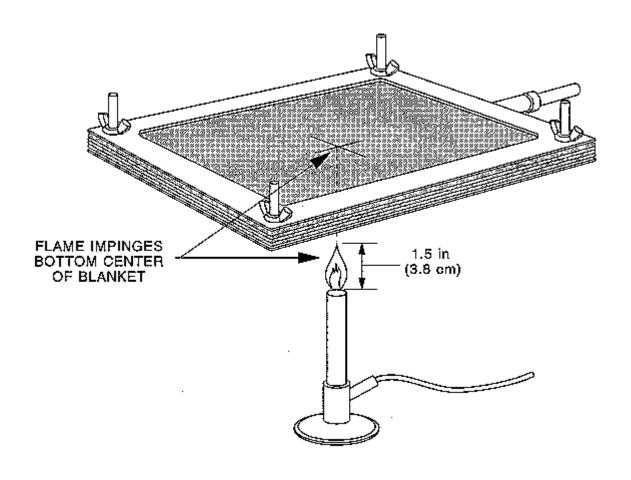
FIGURE B-6. HORIZONTAL TEST FIXTURE WITH 4-PLY BLANKET SAMPLE
